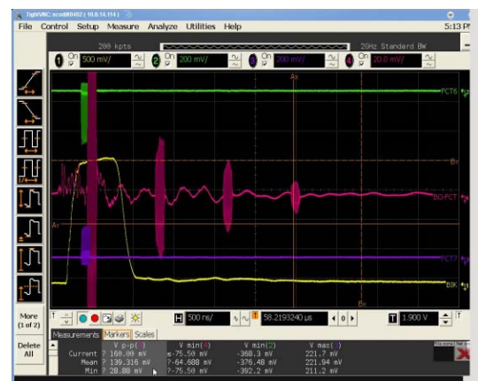
Figure 4: Scope signal with the 2 last FCTs on the transfer line (green and violet traces), kicker pulse (yellow) and the Booster FCT signal (pink trace). The Booster FCT baseline is significantly affected by the kicker pulse.
