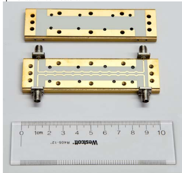
Figure 6: Fabricated board and plates with sma connectors
