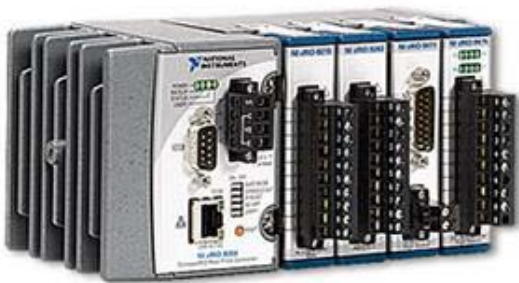
Figure 6: NI CompactRIO, an FPGA hardware platform.
