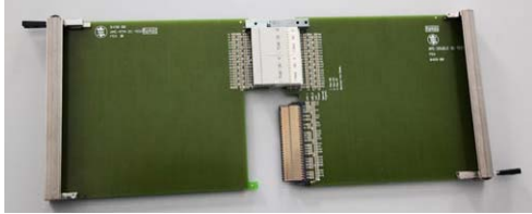
Fig. 9: Double sized AMC “dummy” board with a rear transition module (RTM).
