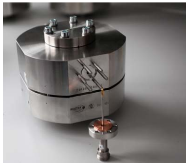
Fig. 11: 1.3 GHz cavity dark current monitor with one coupling antenna in front.
