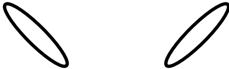
Figure 5. Emittance ellipses for a beam that is focusing and one that is diverging.
