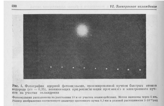
Figure 6: The first photo of hydrogen atoms beam after recombination at NAP-M cooler [6].
