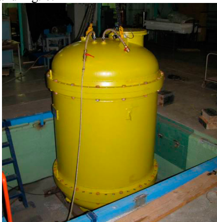
Figure 3: Pressure vessel used for HV section testing.
