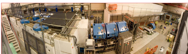
Figure 4: Magnets in MICE beamline (fish-eye lens view)
