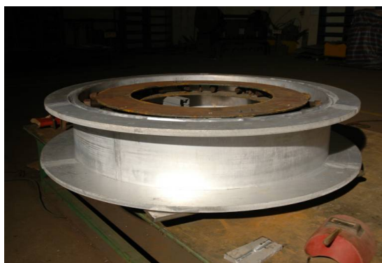
Figure 11: Coil mandrel under welding.
