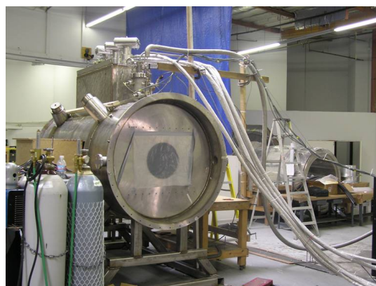
Figure 13: One of the spectrometer solenoid magnets is being tested at the fabrication company.
