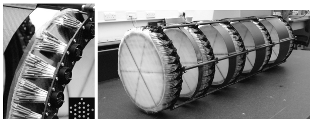
Figure 16: Progress in construction of the scintillating fibers tracker.
