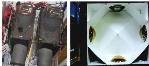
Figure 19: Progress in construction of Cherenkov Counters: CKOVa, CKOVb
