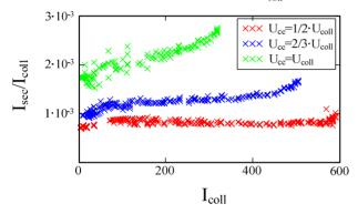
Figure 8: Dependence of efficiency of the collector itself on main beam current.
