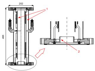
Figure 6: Vacuum chamber of Wien filter.
