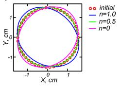
Figure 4: Change of primary beam shape in Wien filter.
