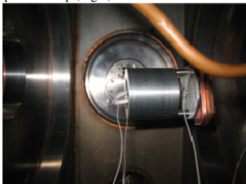
Figure 7. The test electron gun.
