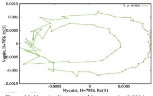
Figure 10: Nyquist diagram, stable case, gain -0.0016.
