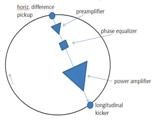
Figure 1: Palmer momentum cooling lay-out.
