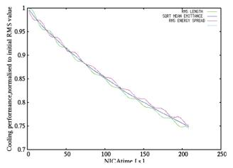
Figure 7: Binning:  $M = 2^{*14}$  bins,  $2^{*13}$  harmonics, 1200 turns, 10 000 sim. ions, gain = -0.0016/turn.
