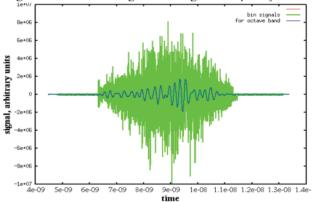
Figure 6: Bunch single passage Green background: signals in the bins, blue: resulting octave (3-6 GHz) stochastic correction signals experienced by passing ions.
