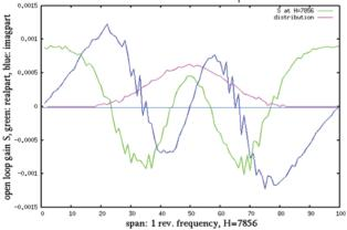
Figure 9:Shows real: green and imag:blue terms of S, using the pu in the position foreseen for NICA (the unwanted mixing is included). Red curve: bunch time-distribution, stable case, gain -0.0016.
