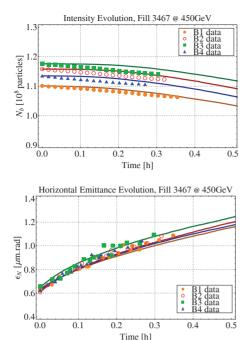
Figure 2: Intensity (top) and emittance (bottom) evolution at injection for 4 single bunches. Dots: measurement, lines: simulation.
