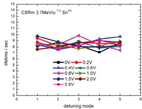
Figure 3: Ion beam lifetime as a function of the modulated mode.
