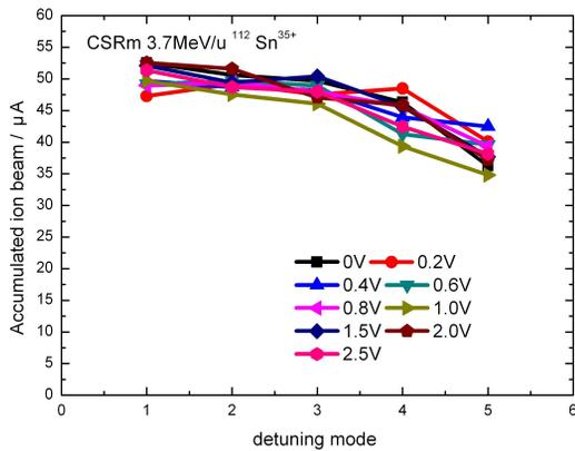
Figure 5: Accumulated ion beam intensity as a function of the modulated mode.
