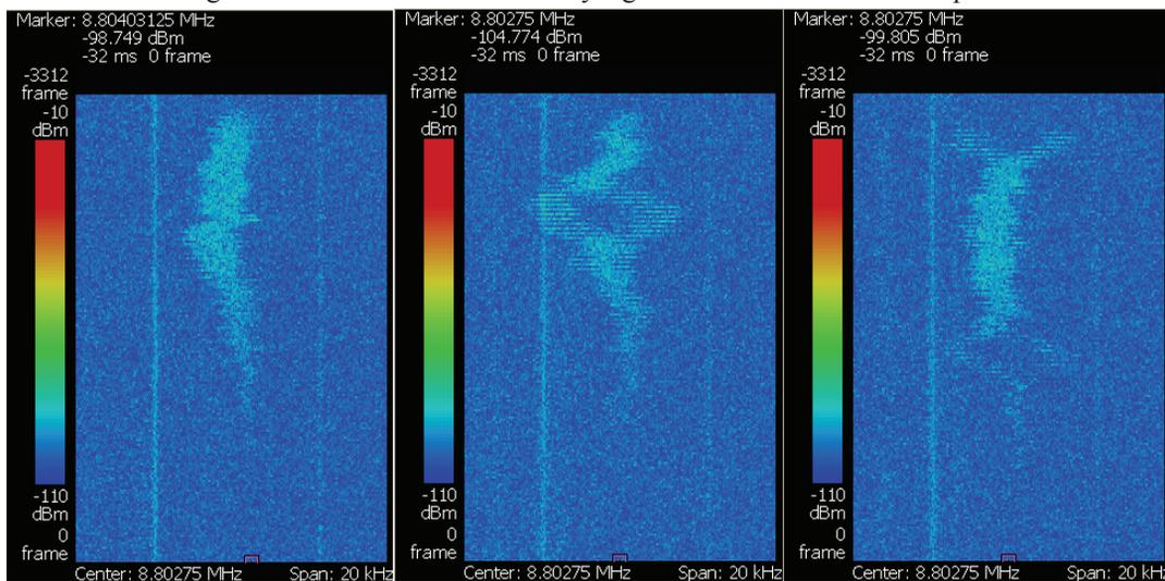
Figure 7: The Schottky signal was splitted into two parts under some modulation The amplitude of modulation was smaller than 2.5V(0.12%).
