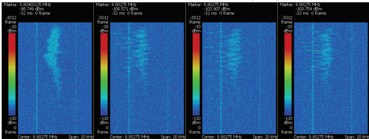
Figure 6: The evolution of Schottky signal with the modulation amplitude.
