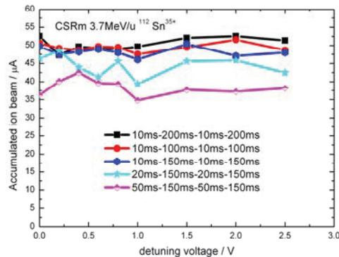
Figure 4: Accumulated ion beam intensity as a function of the modulated voltage.
