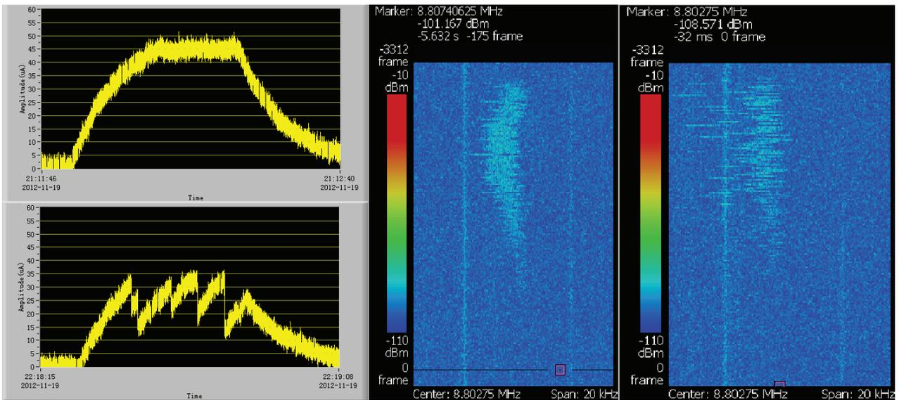
Figure 9: DCCT and Schottky signals at the same time. DCCT signal represents the ion intensity, Schottky signal represents the revolution frequency of ion beam, ion velocity and momentum spread.
