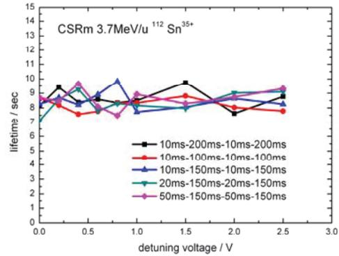
Figure 2: Ion beam lifetime as a function of the modulated voltage.
