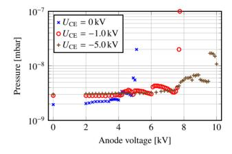
Figure 4: Control electrode voltage dependence of gas discharge effects at  $B_{\parallel} = 200 \,\mathrm{mT}$ .
