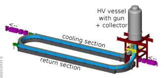
Figure 1: Proposed design of the HESR electron cooler [2].
