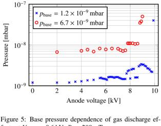
fects at  $U_{CE} = -0.6 \,\text{kV}$ ,  $B_{\parallel} = 200 \,\text{mT}$ .
