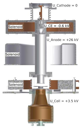
Figure 2: Schematic view of the complete test bench.
