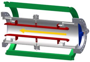
Figure 6: Schematic view of the Wien filter design. Red: electrostatic plates, green: coil for transverse magnetic field, blue: dump for deflected electrons, yellow: primary beam.
