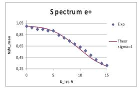
Figure 6: The spectrum of slow positrons.
