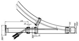
Figure 2: The circulating  $e^+$  beam detector.
