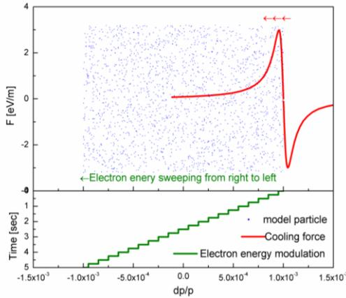
Figure 1: Principle of the electron energy modulation through the ion velocity distribution.
