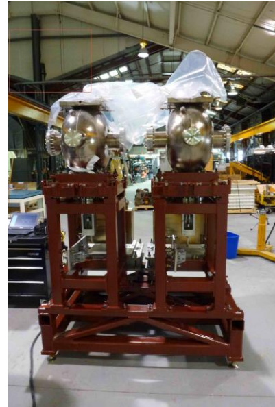
Figure 4: Two 500 MHz cavities mounted on a common support before their installation into the IP2 region.
