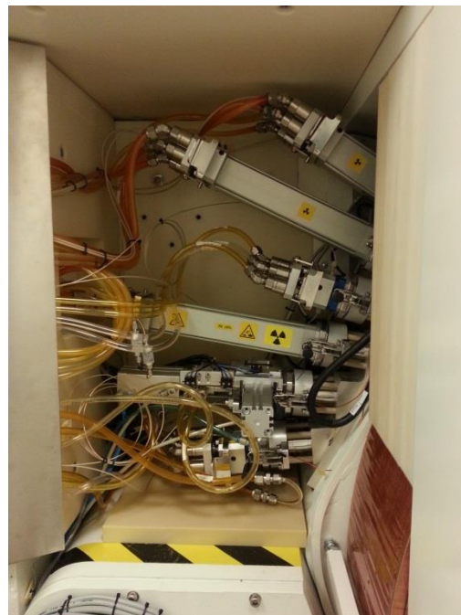
Figure 2: PETtrace target area on locally-shielded cyclotron. The Tc-99m production target is second from the bottom. The transfer tube is obscured by the target station and not visible in the photo.
