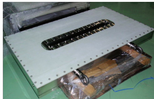
Figure 3: Additional rf cavity to be installed (one half).
