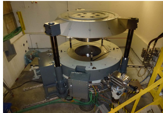
Figure 2: The assembled cyclotron placed in the shielded beam-vault. It can be opened in the median plane as well as at the top of the cryostat. Also visible are the rotoshield (left), the cryocooler-shield (middle) and the vacuum station (right).
