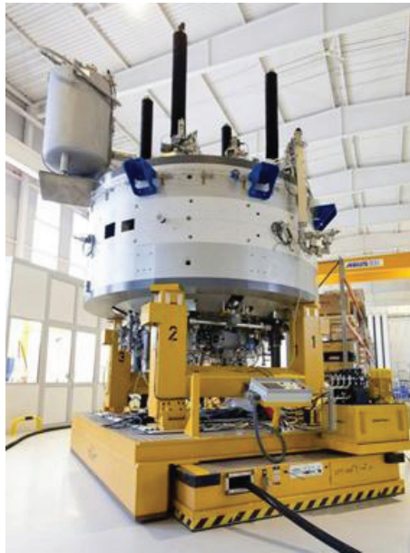
Figure 2: A ProBeam™ cyclotron on its way into the test cell.
