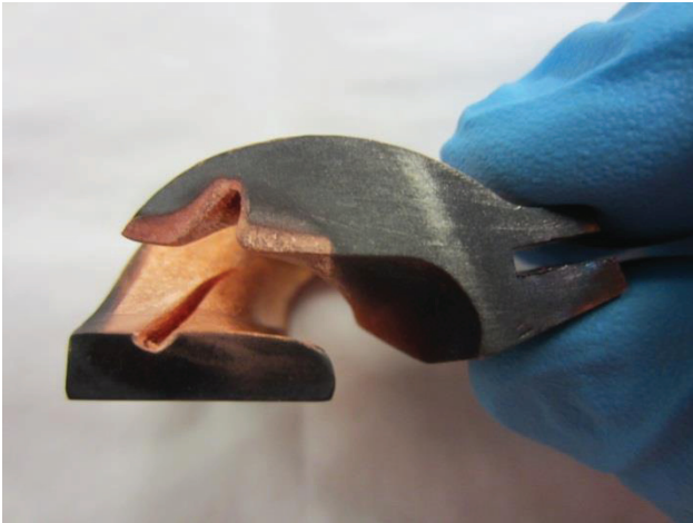
Figure 1: TR30-2 eroded inflector.
