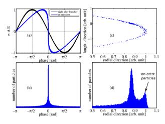
Figure 3: Macroparticle simulation of injection of short bunches: (a) longitudinal phase space right after the first harmonic buncher (black) and right before injection into the cyclotron (blue), in the absence of space charge; (b) phase distribution within the same beam before injection. The same particles, after crossing cyclotron acceleration gap, are show in 'top view' (c), and in radial projection (d).
