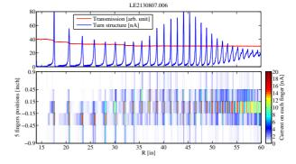
Figure 5: LE2 probe scan showing short bunches injected  $10^{\circ}$  off crest (falling side of the rf wave). (See caption of Fig. 4 for plot details.)
