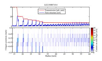
Figure 6: LE2 probe scan showing short bunches injected  $-10^{\circ}$  off crest (rising side of the rf wave). (See caption of Fig. 4 for plot details.)
