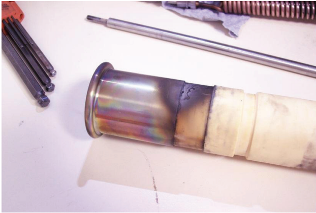
Figure 6: Damage on deflector insulator.
