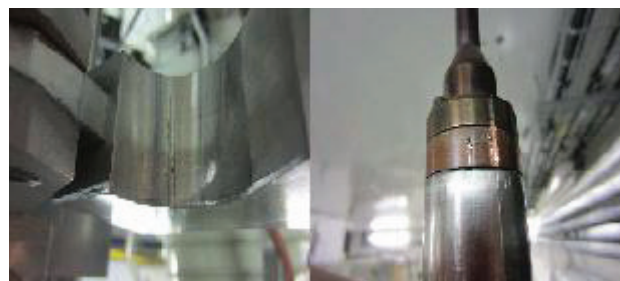
Figure 5: Damage on the guidance system of the ion source (left) and stripe on the shaft (right).
