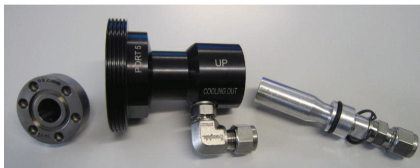
Figure 9: New conical design [2]: Niobium insert, target body, one piece water diffuser.
