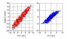
Figure 5. The horizontal and vertical emittances of the extracted beam (A/Z=8, Bo=1.45 T)
