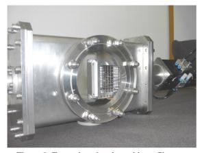
Figure 9. Extraction chamber with profilometer
