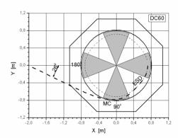
Figure 1. Trajectory of the test ion (A/Z=8, Bo=1.45T) extracted from DC60 cyclotron
