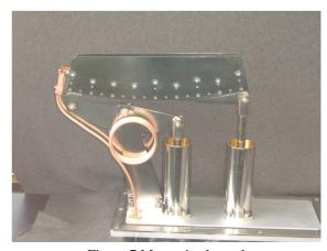
Figure 7 Magnetic channel
