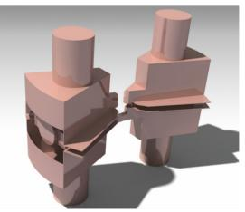
Figure 6: Final RF cavity design using CATIA V5
