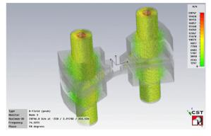
Figure 5: Magnetic field distribution
