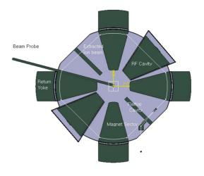
Figure 2: Separated Sector magnet Layout
