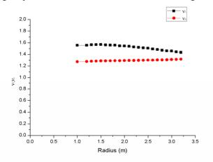
Figure 9: Radial and Axial beam tunes
