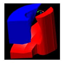
Figure 6: Inflector with the "bended" electrodes.
