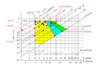
Figure 4: Acceleration performance of the RIKEN AVF cyclotron.
