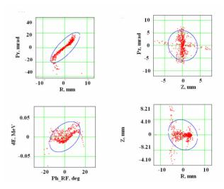
Figure 3: Beam emittance at the final radius, upstream of the deflector.
