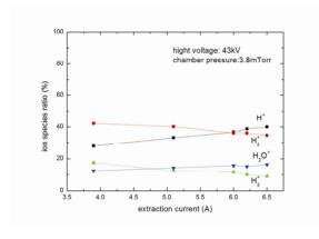
Figure 4: Proton ratio as a function of extraction current
