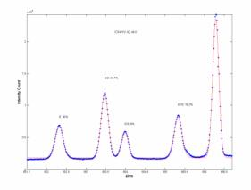
Figure 3: Spectrum of the H<sub>a</sub> lines of ion beam
