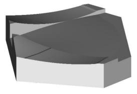
Figure 4: Modified pole face of the analyzing magnet  $\odot$  with parabolic shapes to compensate the second-order  $\Xi$  aberrations.
