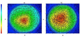
Figure 2: CCD images in false colours of an Ar plasma at the extraction region of the source. In a) the biased disk voltage is -200 V and the extracted  $Ar^{8+}$  current is 450  $\mu$ A, while in b) the disk floats at -60 V and the extracted  $Ar^{8+}$  current is only 200  $\mu$ A.
