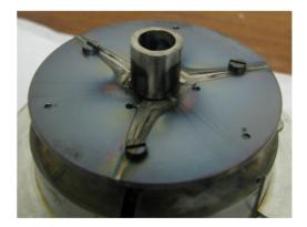
Figure 1: The plasma electrode with its collar.
