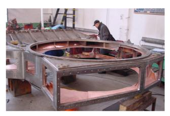
Figure 1: SFC double-deck vacuum chamber
