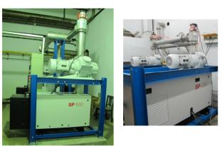
Figure 3: The new rough pumping stations of SSC and SFC
