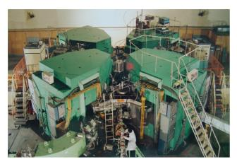
Figure 2: SSC (vacuum chamber is between the magnets)
