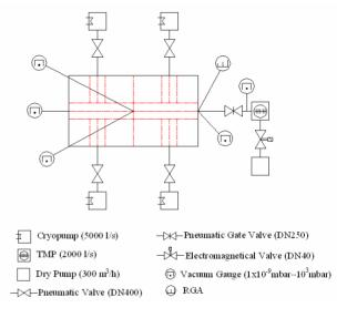
Figure 4: The vacuum equipment layout of the cyclotron
