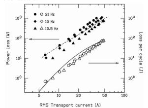
Figure 3: Measured AC losses at 20K of the Bx coils in series. Full symbols show the total power losses on the left side scale. Open symbols present losses per cycle on the right side scale. The dashed curve shows the model calculation by King [11]. The solid curve is a theoretical prediction normalized to the measured data.
