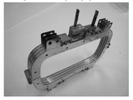
Figure 2: Photograph of single assembled Bx coil.
