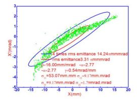
Figure 3: Horizontal emittance
