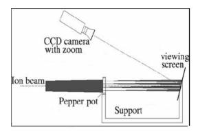
Figure 5: The scheme of the pepper-pot system
