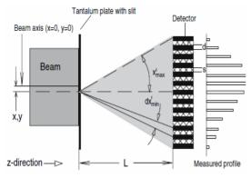
Figure 3: Scheme of slit-grid system
