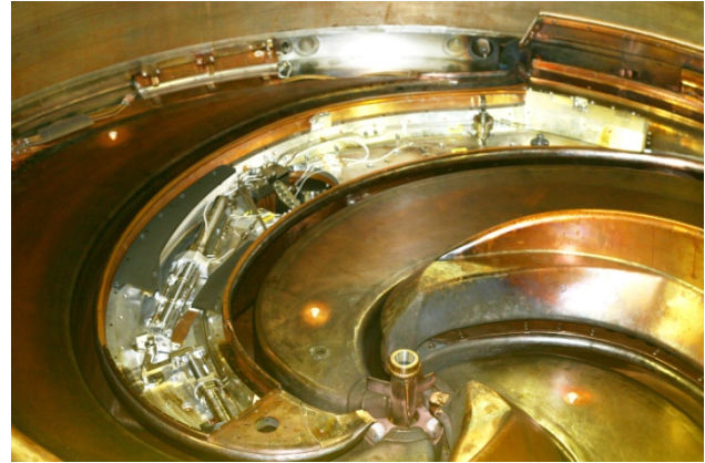
Figure 2 K1200 cyclotron. The upper half of the dee has been removed, as well as the RF shield that covers the stripper mechanism. The platter with the chain that drags the stripper foil holders has also been removed. The water cylinders used to drive the platter and locate the platter in the correct position are shown.
