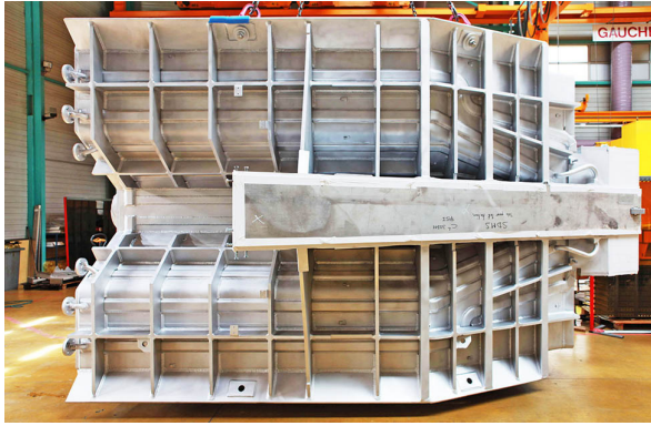
Figure 8: The first one of two new resonators for the Injector II, delivered by the French company SDMS.
