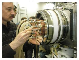
Figure 6: Sergey Grigorenko, NIIEFA, shows how to change the filament in the ion source.
