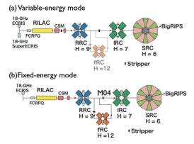
Figure 1: Acceleration schemes used in RIBF.
