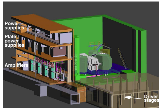
Figure 8: Layout of Injector II with new building for power amplifiers on the left.
