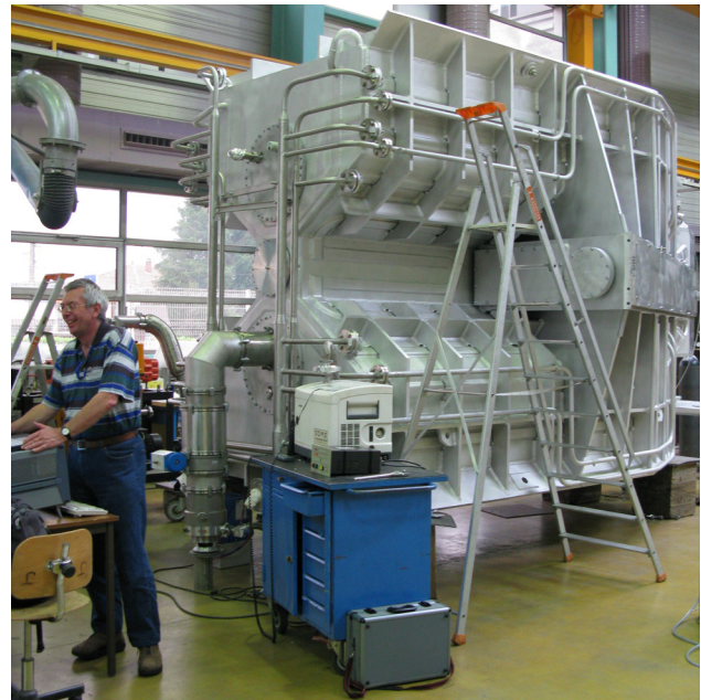
Figure 7: LLRF-measurements of new 50MHz prototype resonators for the Injector II cyclotron at SDMS.
