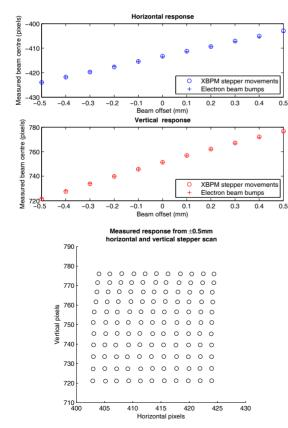
Figure 5: First position measurements made using the Aperture XBPM.
