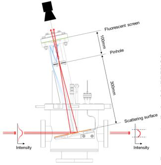
Figure 4: Schematic of scattering optics. The pinhole and the fluorescent screen are in-vacuum, and visible light from the screen is viewed with a GigE camera through an optical viewport. The red lines show the expected path of the Xrays, scattered by the surface of the copper aperture. The blue lines show the likely path that the visible light was taking through the vent holes inside the XBPM.
