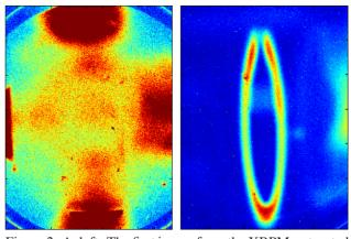
Figure 3: A, left: The first image from the XBPM, saturated by visible and UV light. B, right: The image seen after baffles and larger pinhole were installed. Both show the EPU64 at 16mm gap and circular phase.
