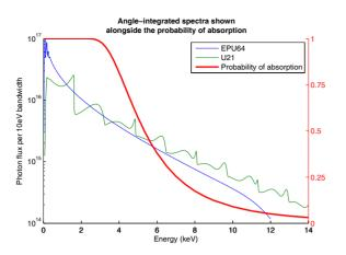
Figure 2: Shown is the integrated spectra of the I06 EPU64, circular phase and 16mm gap, and an in-vacuum U21 at 5mm gap. The U21 spectra contains more photons at high energies, but the EPU64 has more photons at low energies where they are more readily absorbed. The calculated absorption rate for a 200µm thick carbon foil is shown.
