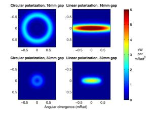
Figure 1: The beam intensity and distribution varies between polarisations and gaps.
