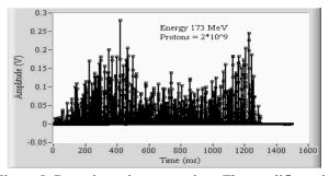
Figure 5: Beam intensity versus time. The amplifier gain is G5 and the acquisition rate is 10 kHz.
