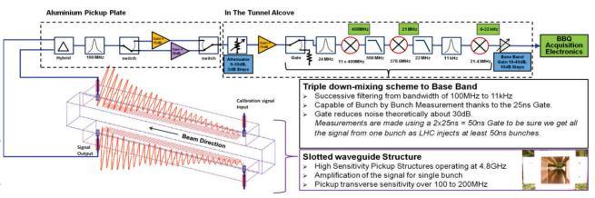
Figure 1: The Analogue Processing Chain.
