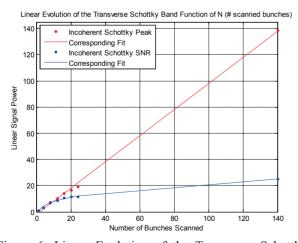
Figure 6: Linear Evolution of the Transverse Schottky peak (red) and of the SNR (blue).
