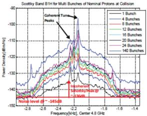
Figure 5: Incoherent Schottky Bands for protons at Collision.
