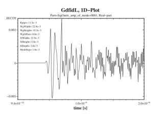
Figure 3: Signal coupled into a waveguide through a rectangular window in the beampipe.
