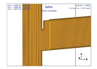
Figure 1: A rectangular waveguide coupling to the beampipe through a rectangular slot.
