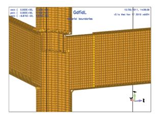
Figure 5: A modified geometry with the coupling slot sunk into the beampipe for increased coupling.
