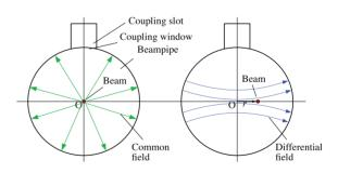
Figure 2: A rectangular waveguide coupling to the beampipe through a rectangular slot.
