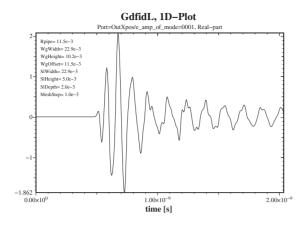
Figure 6: Signal coupled by a sunken slot.
