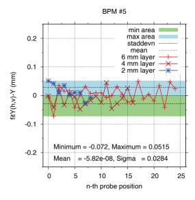
Figure 5: Difference between reconstructed and real probe position.
