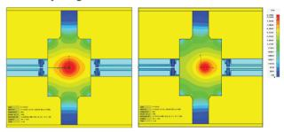
Figure 5: E-fields of a centred (left) and an offset (right) nominal bunch passing between the buttons A and B.
