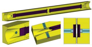
Figure 2: Cross-sections of the collimator "Demonstrator"
