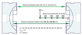
Figure 7: Schematic for the beam "horizontal sweep" simulations.
