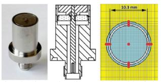
Figure 3: Photograph and a meshed model of the  $\emptyset$  10 mm stainless steel button BPM.
