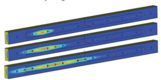
Figure 6: E-fields of a centred bunch with  $\sigma$  of 125, 250 and 500 ps.
