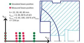
Figure 10: Schematic for the beam "area sweep" simulations.
