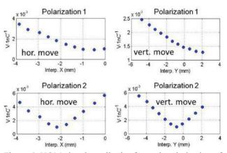
Figure 6: HOM signal amplitudes for each polarization of the beampipe mode of cavity 2 as a function of the beam position interpolated in the cavity.
