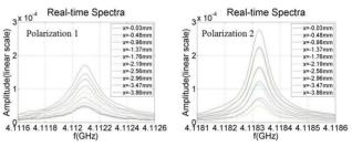
Figure 5: Frequency-domain signals of the beampipe modes from the first dipole passband measured from HOM coupler C2H2.
