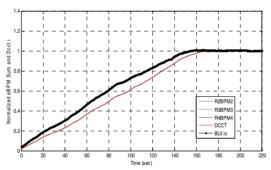
Figure 7: photon intensity, BPM sum value and beam current change during injection from zero to 360 mA.
