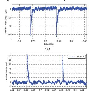
Figure 2: (a) Storage Ring electrical R1BPM4 10kHz readings during injection (b) Beamline 10 photon BPM 10 kHz rate reading during injection.
