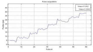
Figure 5: Wire movement – by 5 um steps in X-direction. Seven steps are seen in position measurement.
