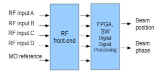
Figure 1: Libera Single Pass H block diagram.
