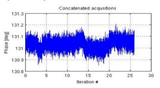
Figure 4: Negligible impact of the off-centred beam on the phase measurement.
