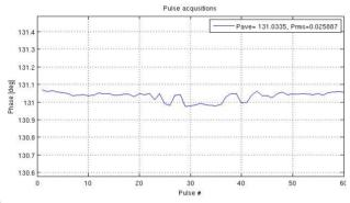
Figure 6: Impact of the off-centred beam on the phase measurement.
