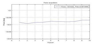
Figure 8: Consecutive macro pulse acquisition – phase measurement.
