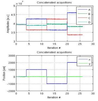
Figure 3: Wire movement measurement. Concatenated results for the displacements over a larger scale (X = +1 mm, -1 mm, +2 mm; Y = 0 mm). Four amplitudes and X, Y positions are plotted.
